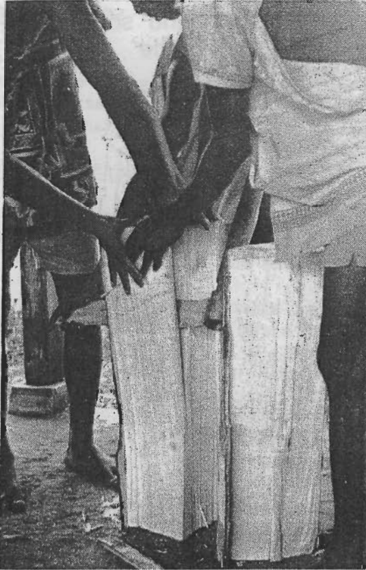
Figure 5 Splitting Shakes with the Froe
