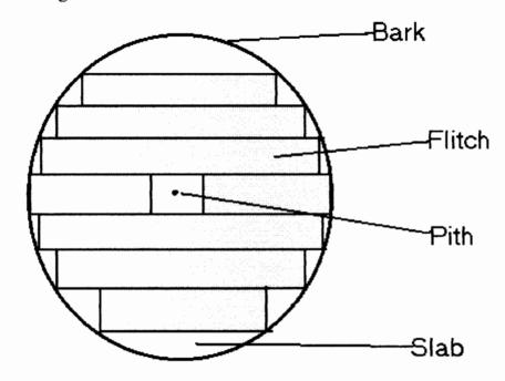
Note: A flitch is free from wane and pith and must measure more than  $150 \text{mm} \times 150 \text{mm}$ .
